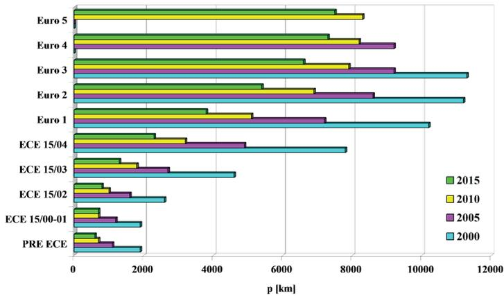
Fig. 3. Average annual mileage of passenger cars with spark-ignition engines of (1.4÷2) dm<sup>3</sup> cubic capacity, classified in ecological categories
